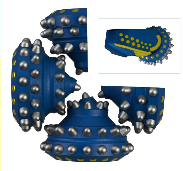
Designed for medium hard to hard abrasive formations; hard copper ores, hard sandstone, medium hard iron ore, schist, gneiss, metamorphic formations; granite and medium hard igneous. USC: 15,000 to 44,200 PSI (103 to 305 Mpa)
