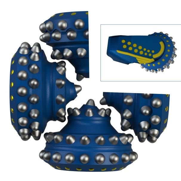
Designed for hard and very abrasive formations; hard copper ores, hard iron, quartz and the hardest igneous formations.
