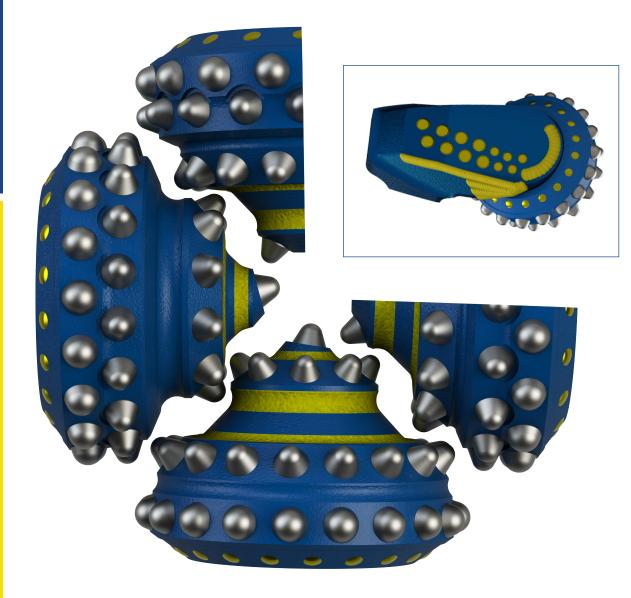
Designed for hard and very abrasive formations; hard copper ores, hard iron, quartz and the hardest igneous formations. USC: 30,000 to 60,000 PSI (207 to 414 Mpa)
