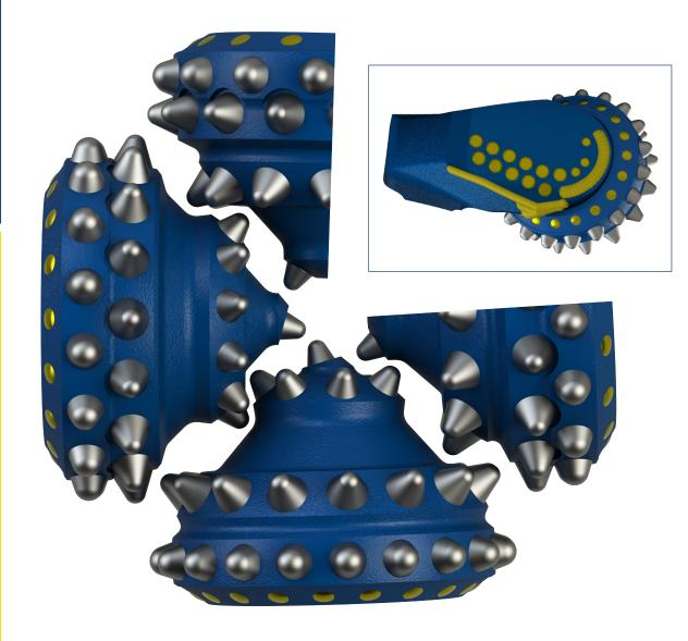
Designed for medium to medium hard formations including sulfide and oxide copper ores, soft iron formations, medium-hard sandstone, dolomite and limestone. USC: 8,000 to 30,000 PSI (55 to 207 Mpa)
