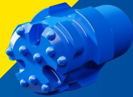
Forepoling ring bit system and casing tubes are designed to be drilled with top hammer or DTH in an umbrella shape as secondary support in the tunnel roof. Weak ground and overburden must be strengthened by grouting through the casing and grouting valves into the ground.
