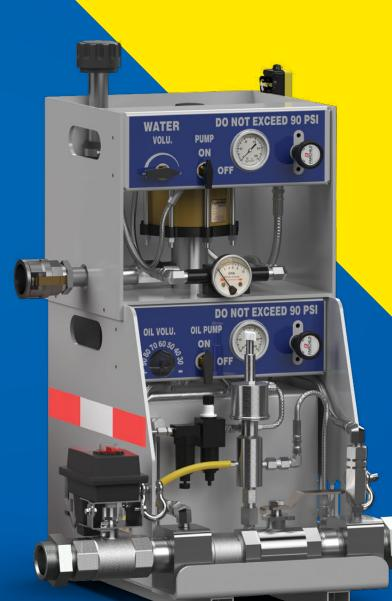
Optional add-on fluid injection system delivers a mixture of water, foam, and/or polymer at a rate of 0-5 gal/min (0-19 l/min) into the air-stream, assisting with dust suppression, lubrication, and removal of cuttings.
