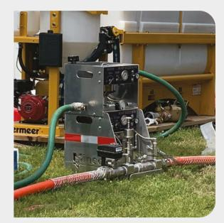
Optional add-on fluid injection system delivers a mixture of water, foam, and/or polymer at a rate of 0-5 gal/min (0-19 l/min) into the air-stream, assisting with dust suppression, lubrication, and removal of cuttings.
