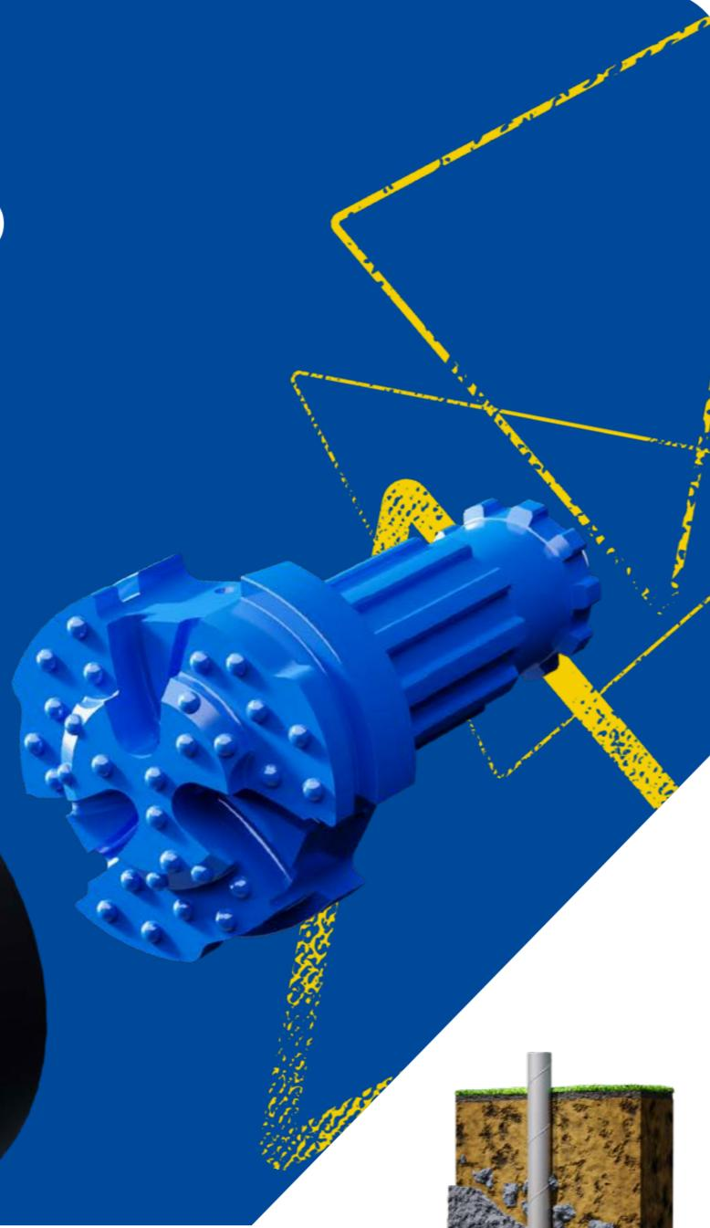
**Integrated ring bit systems**, divided into small and large designs, are designed for drilling end-bearing piles through overburden into bedrock. The system can drill straight and inclined piles through boulders and rock layers and it easily manages situations where the bedrock itself is inclined.
