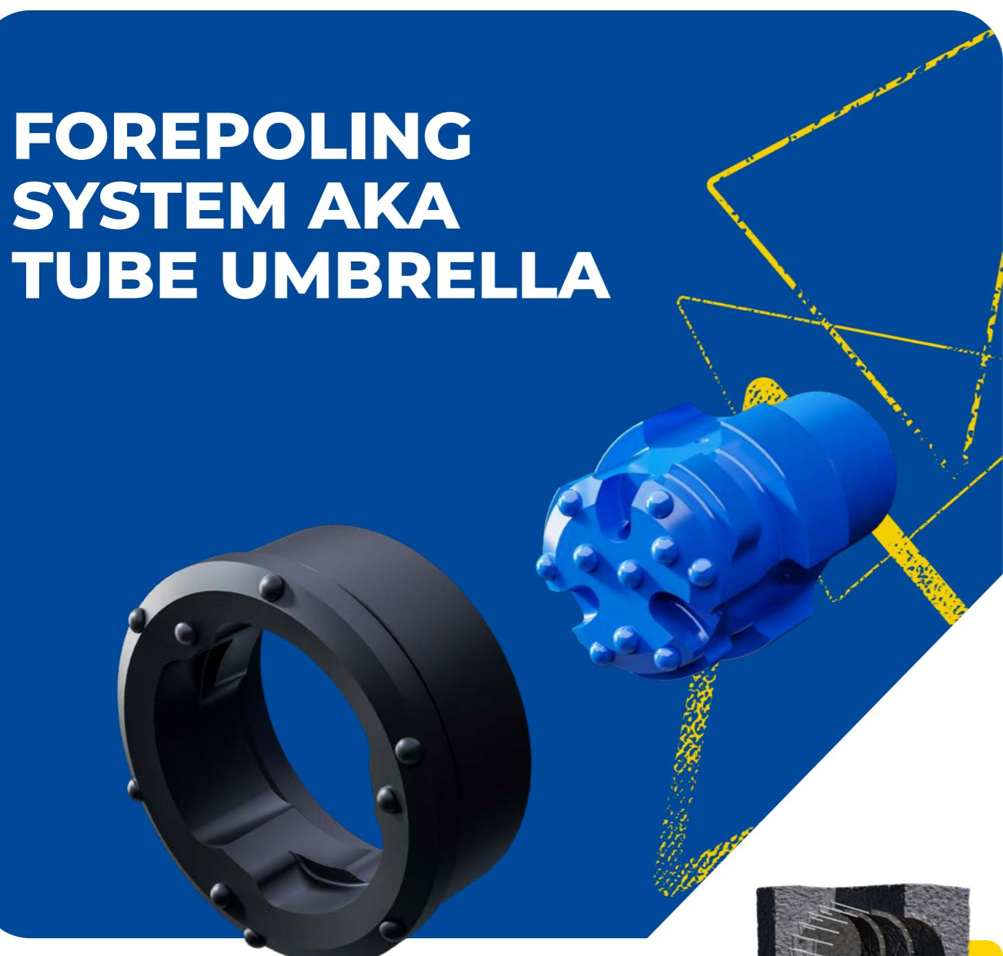
**Forepoling ring bit system and casing tubes** are designed to be drilled with top hammer or DTH in an umbrella shape as secondary support in the tunnel roof. Weak ground and overburden must be strengthened by grouting through the casing and grouting valves into the ground.
